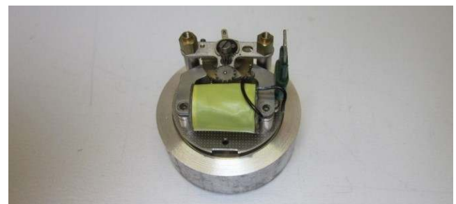
Above: Photo 2 - The clock as removed from the Rev Counter ready to be modified. Below: Photo 3 -The clock with back and setting stem removed.
