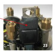
23. If the top of the plastic insulating sleeve is damaged, cover the damaged part with the heatshrink sleeving supplied and use a hair dryer or heat gun to shrink the sleeving over the plastic insulating sleeve.
