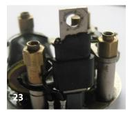
Heat-shrink sleeving shrunk over damaged insulating sleeve
