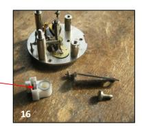
15. Undo connecting bracket retainer screw and remove connecting bracket and plastic support. Note that the plastic connecting bracket support is no-longer required and should not be refitted.
