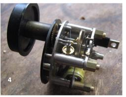
4. Remove back-plate to leave the movement as shown on right. If the back-plate is stiff to remove it may be necessary to gently lever it with a small screwdriver
