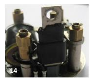
Heat-shrink sleeving shrunk over damaged insulating sleeve
