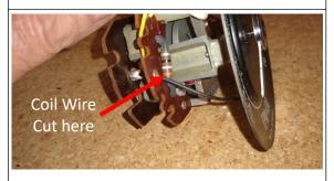
Fitting Instructions for Smiths RVI Type Tachometers (later 'Gen 2' type with bullet connectors)
