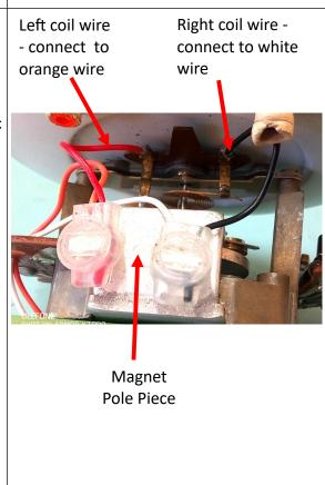
Fitting Instructions for Smiths RVI Type Tachometers (later 'Gen 2' type with bullet connectors)
