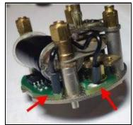
I took the opportunity to remove the old electrical tape around the solenoid and put new tape on it – beware though when doing this not to break the wiring under the tape.
